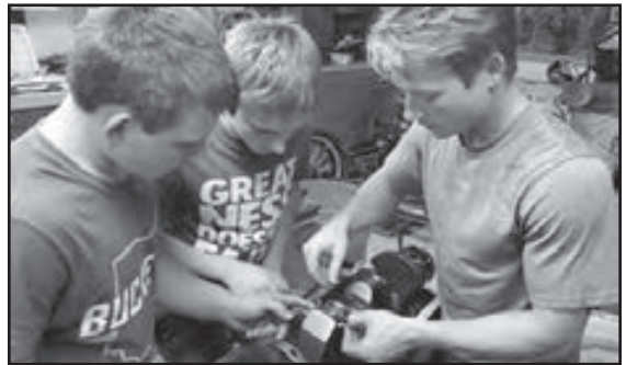
Brad, Darren, and Travis install the shims for the connecting rod.
