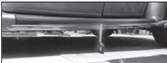
Original running board trim has a slight dip in it.
