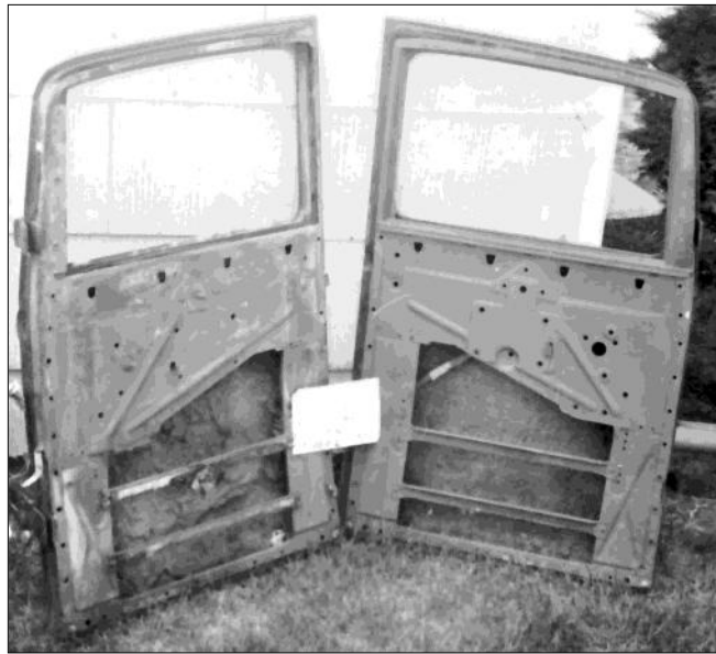
Early (left) and late Fordor inner door panels
